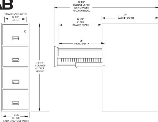
Fire, Impact and Explosion Rating The Schwab Series 5000 vertical file has met Underwriters' Laboratories stringent requirements for the classification of 'Record Protection Equipment.' This includes a test for fire-resistance in external temperatures exceeding 1700°F for one hour, a 2000°F explosion hazard test as well as a test to withstand the impact of a 30 ft. drop.
